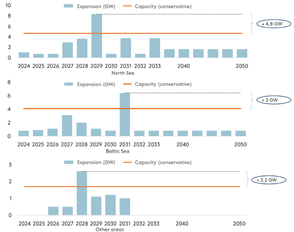
Figure 2.5: Bottlenecks in the North Sea, Baltic Sea and other areas, divided by investments in upgrades of quay bearing capacity and channel depth in all Danish installation ports, (GW).
